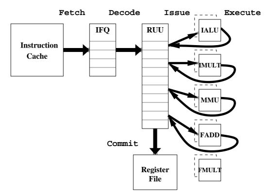
Figure 4.1: Datapath of basic microprocessor.
