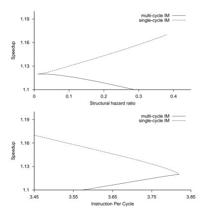
Figure 5.1: Comparison of single to multi-cycle IM. On a large pipeline machine the number of FUs is raised until the structural hazard ratio is 0. Speedup is shown as a function of the structural hazard ratio and of IPC.
