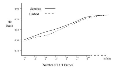
Figure B.4: Hit ratios as a function of LUT size (set size is 4). MEMO-TABLE is unified (dashed line) or separate MEMO-TABLES are used (solid line).
