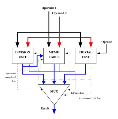
Figure 3.3: Layout of a Trivial Test Unit adjacent to a MEMO-TABLE and Division Unit.
