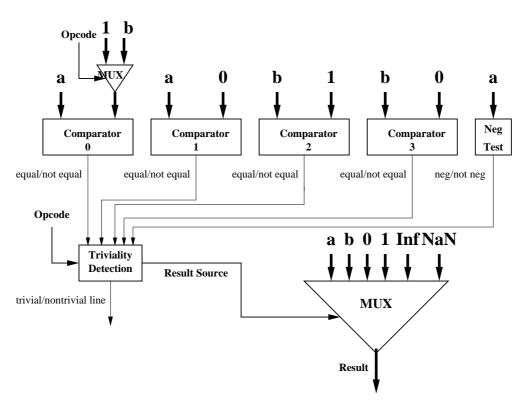
Figure 3.4: Layout of a Trivial Test Unit, the opcode of the instruction determines which comparisons are used.
