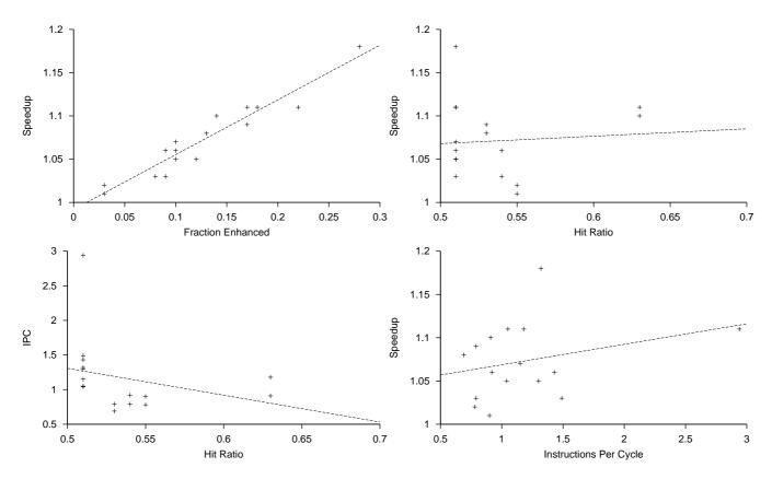
Figure 4.5: Correlations between FE and speedup (upper-left), hit-ratio and speedup (upper-right), hit-ratio and IPC (lower-left), IPC and speedup (lower-right).
