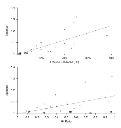
Figure 4.3: Correlation between FE to speedup and between hit-ratio to speedup (integer applications are circled). Lines are best fit using the Marquardt-Levenberg algorithm.
