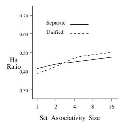
Figure B.5: Hit ratios as a function of set associativity size. MEMO-TABLE is unified (dashed line, 512-entry) or separate MEMO-TABLES are used (solid line, 256-entry per MEMO-TABLE).
