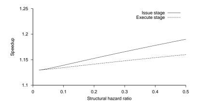
Figure 4.6: Comparison of IM in the issue and execute stages. On a large pipeline machine the number of FUs is raised until the structural hazard ratio is 0. Speedup is shown as a function of the structural hazard ratio.
