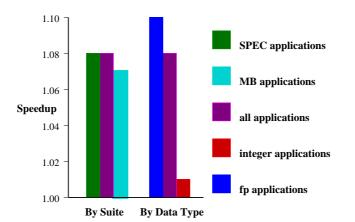
Figure 4.4: Breakdown of speedup by application suite (SPEC, MediaBench) and by data type (FP, Int).
