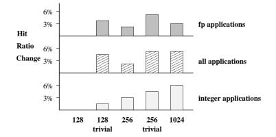
Figure 3.5: Changes in hit-ratio of MEMO-TABLES with and without trivial calculation detection (base MEMO-TABLE of size 128/4).
