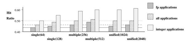
Figure 3.6: hit-ratio of single, multiple, and unified contents scheme. Each MEMO-TABLE is 4-way set associative, uses random replacement, uses the LSBs of the operands (and opcodes) as indices to MEMO-TABLE entries, and performs trivial calculation detection.
