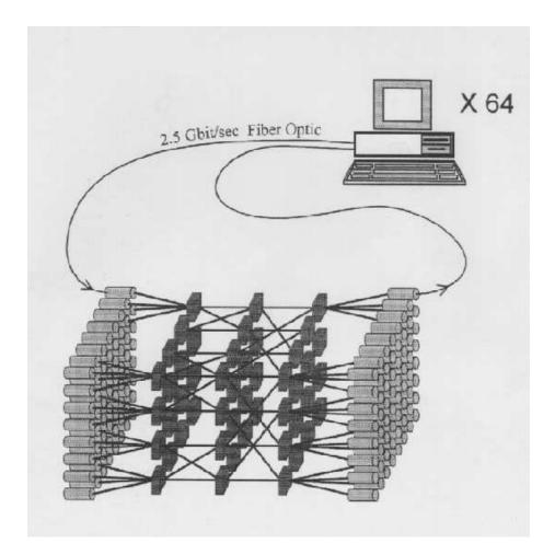
Figure 2.4: Example for building the switch with a multi stage topology
