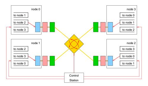
Figure 2.3: The configuration when node i sends to node i + 2
