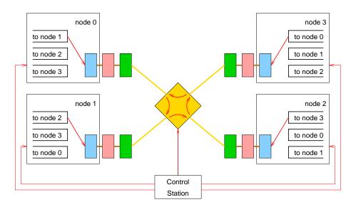
Figure 2.2: The configuration when node i sends to node i + 1
