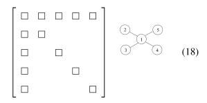
with cliques  $C_1 = \{1,2\}, C_2 = \{1,3\}, C_3 = \{1,4\}$  and  $C_4 = \{1,5\}$ . A typical signal processing application is a wireless network in which the global node is the access point and the local nodes are the terminals. Other applications of these models are discussed in [40].
