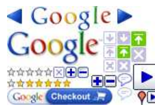
Figure 1. Composite image containing multiple graphical elements used to render the Google search results page
