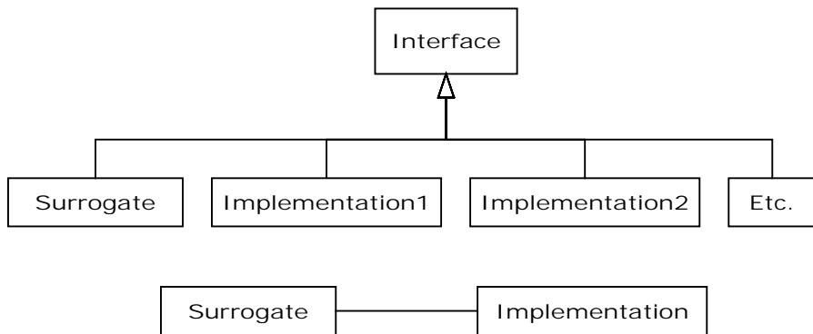
When a surrogate object is created, it is given an implementation to which to send all of the method calls.
