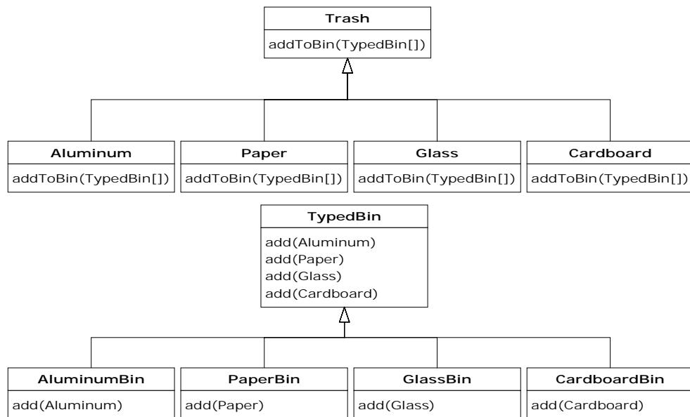
The new hierarchy is **TypedBin**, and it contains its own method called **add()** that is also used polymorphically. But here's an additional twist: **add()** is *overloaded* to take arguments of the different types of trash. So an essential part of the double dispatching scheme also involves overloading.
